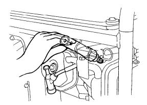
7. After each spark plug is seated, tighten with a spark plug wrench to compress the washer.
