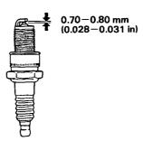
6. Check that the spark plug washer is in good condition, and thread the spark plug in by hand to prevent cross-threading.
