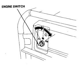
6. When the engine starts, allow the engine switch to return to the ON position
