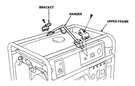
NOTE: Install at near center avoiding to install over the fuel filler cap.
