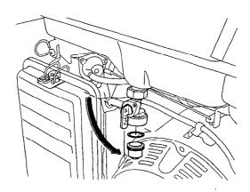
d. Drain the carburetor by loosening the drain screw. Drain the gasoline into a suitable container.
